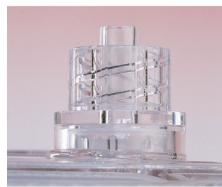
The device has a bubble trap that includes a filter screen to deflect bubbles up to the membrane, which then vents the air out of the system.
